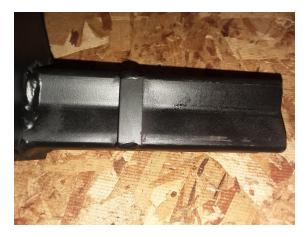
The tops of your Caster set have welded "stop tabs" to ensure proper placement.
