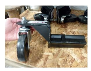
The swivel casters are designed to roll into place when the lift is being raised.
