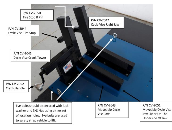
The CV-2049 Cycle Vise is designed to mount directly to all HMC Lift Tables. It is secured to the table using 10 sets of 5/16-18 x 3/4" Hex Bolt, Lock Washer, & Nut. To accommodate wide front tires, P/N CV-2045 may be mounted on the outside four holes. In this case, the 3/8-16 Eye Bolt must be used as 1 of the fasteners. The Vise can be mounted in two locations to accommodate longer or shorter wheel bases. For long wheel base bikes mount the Cycle Vise all the way forward.
